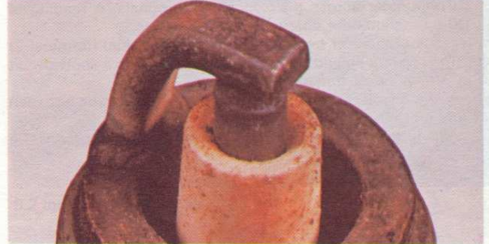
Overheating. Electrodes have glazed appearance, core nose very white – few deposits. Fault: plug overheating. Check: plug value, ignition timing, fuel octane rating (too low) and fuel mixture (too weak). Discard plugs and cure fault immediately
