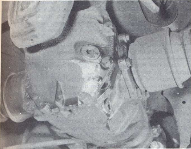
5.2 Final drive unit showing filler and drain plugs
