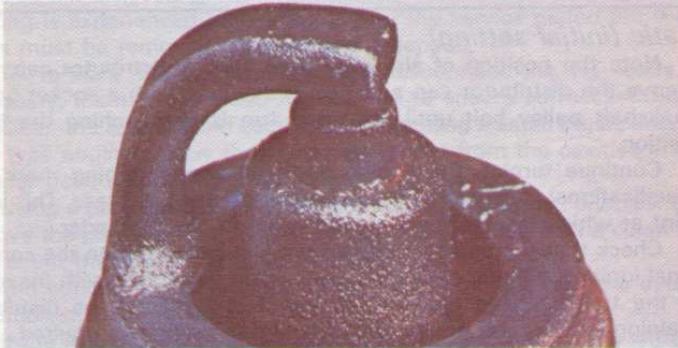
Oil fouling. Wet, oily deposits. Will cause weak spark and eventually misfire. Fault: worn bores/piston rings or valve guides; sometimes occurs (temporarily) during running-in period. Plugs can be re-used after thorough cleaning
