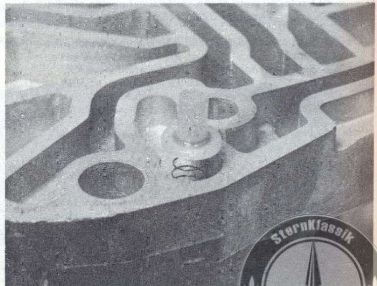
17.10B One-way throttle valve location in bottom housing
