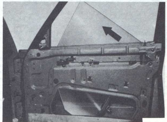
Fig. 12.10 Removing the front door window (Sec 17)
