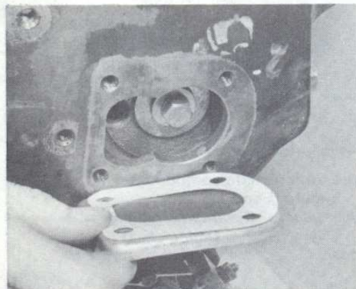
12.5 Removing the intermediate gear cover plate (123 engine)
