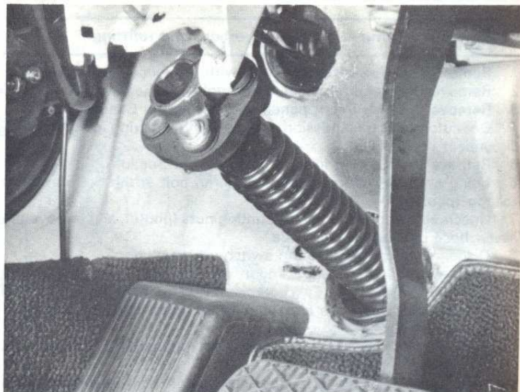
23.4 Steering column safety corrugated tube
