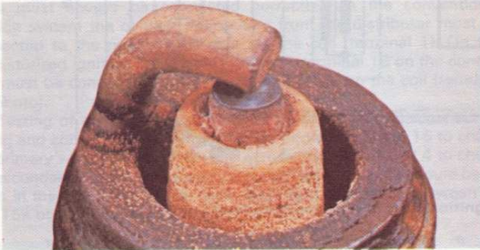
Normal. Grey-brown deposits, lightly coated core nose. Gap increasing by around 0.001 in (0.025 mm) per 1000 miles (1600 km). Plugs ideally suited to engine, and engine in good condition
