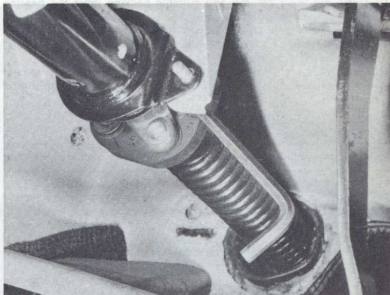
21.6 Removing the steering column lower clamp bolt
