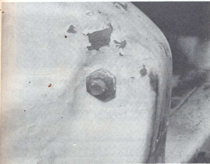
9.4 Front upper control arm inner pivot bolt
