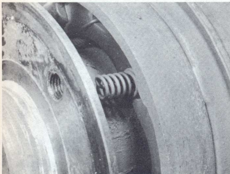
12.4 Shoe steady spring location for the handbrake/parking brake
