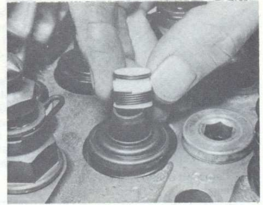
10.4A Removing an inlet valve stem seal (123 engine)
