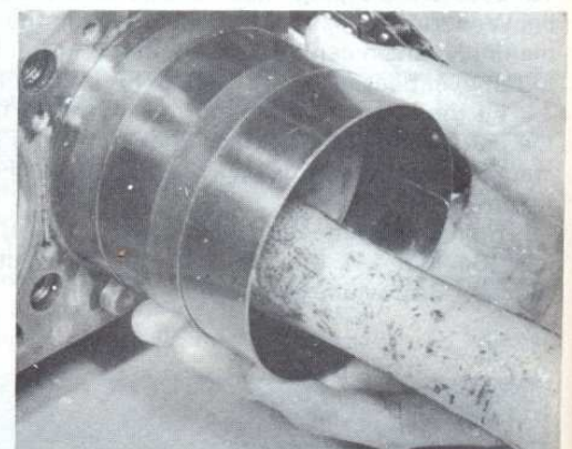
32.4B ... and drive the piston into the cylinder with the handle of a hammer
