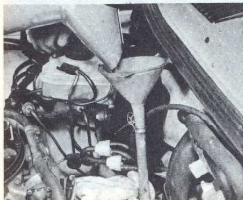
11.4 Topping-up the automatic transmission fluid
