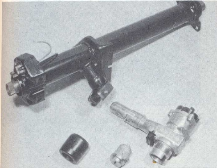
23.9 The steering lock removed from the steering column
