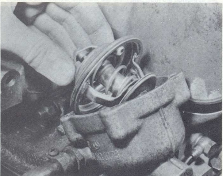
7.4 Withdraw the thermostat
