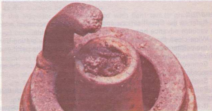
Electrode damage. Electrodes burned away; core nose has burned, glazed appearance. Fault: pre-ignition. Check: as for 'Overheating' but may be more severe. Discard plugs and remedy fault before piston or valve damage occurs
