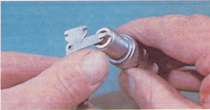
Measuring plug gap. A feeler gauge of the correct size (see ignition system specifications) should have a slight 'drag' when slid between the electrodes. Adjust gap if necessary
