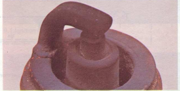
Carbon fouling. Dry, black, sooty deposits. Will cause weak spark and eventually misfire. Fault: over-rich fuel mixture. Check: carburettor mixture settings, float level and jet sizes; choke operation and cleanliness of air filter. Plugs can be re-used after cleaning
