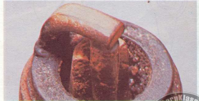
Split core nose (may appear initially as a crack). Damage is self-evident, but cracks will only show after cleaning. Fault: pre-ignition or wrong gap-setting technique. Check: ignition timing, cooling system, fuel octane rating (too low) and fuel mixture (too weak). Discard plugs, rectify fault immediately
