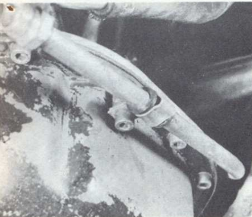
5.12C Oil cooler pipe left-hand side bracket (automatic transmission models)
