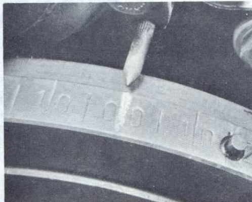
5.4B Ignition timing pointer aligned with TDC mark on the vibration damper
