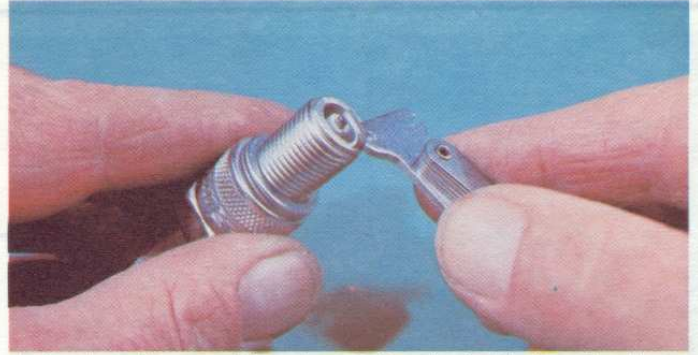
Adjusting plug gap. The plug gap is adjusted by bending the earth electrode inwards, or outwards, as necessary until the correct clearance is obtained. Note the use of the correct tool
