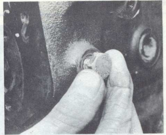
12.11 Removing the timing chain limit pin (123 engine)
