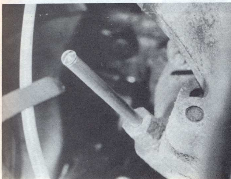
8.1 CO meter take-off point on the exhaust manifold
