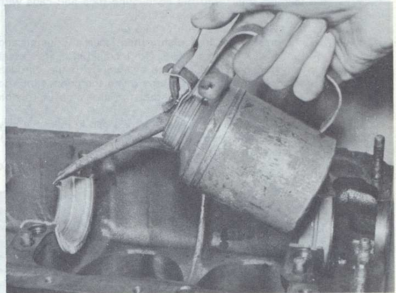
31.3 Lubricating the main bearing upper shells
