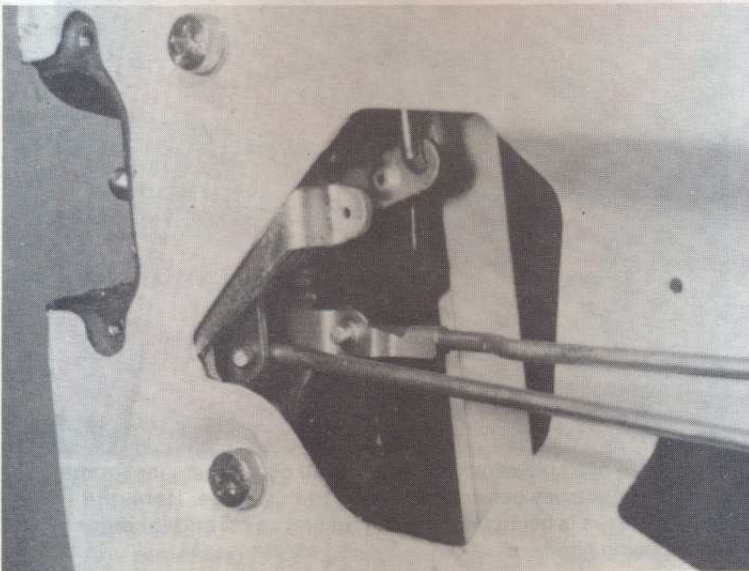
24.2B Operating rods on the front door lock
