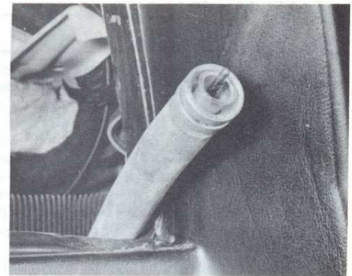
18.5B Square section end to the speedometer cable
