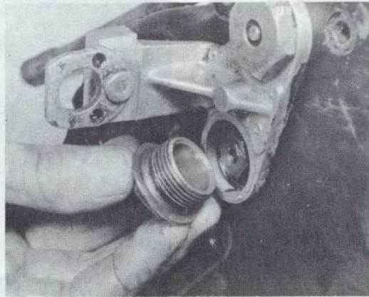
17.4A Unscrew the plug ...
