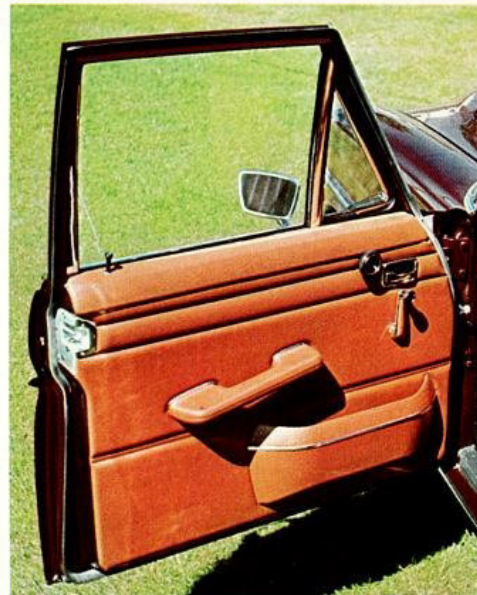
Door handle is recessed for passenger protection. Pocket keeps maps at your fingertips.
