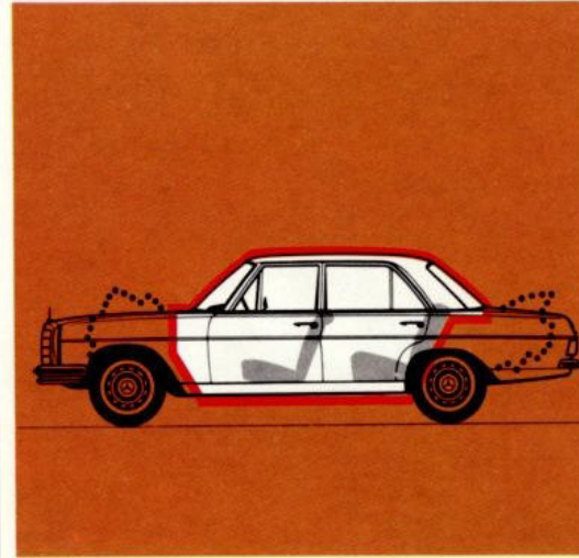
Diagram showing the distortion principle: rigid passenger compartment but energy-absorbing, collapsible front and rear sections.
