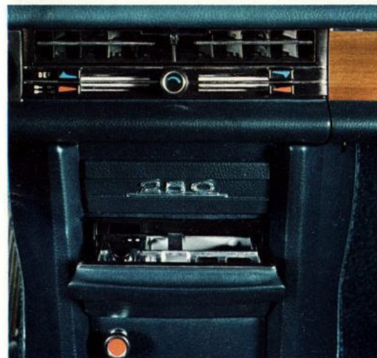
Effective heating and ventilation system, providing any degree of hot or cold air, upwards or downwards, right or left. Above: a very large adjustable fresh air duct.
